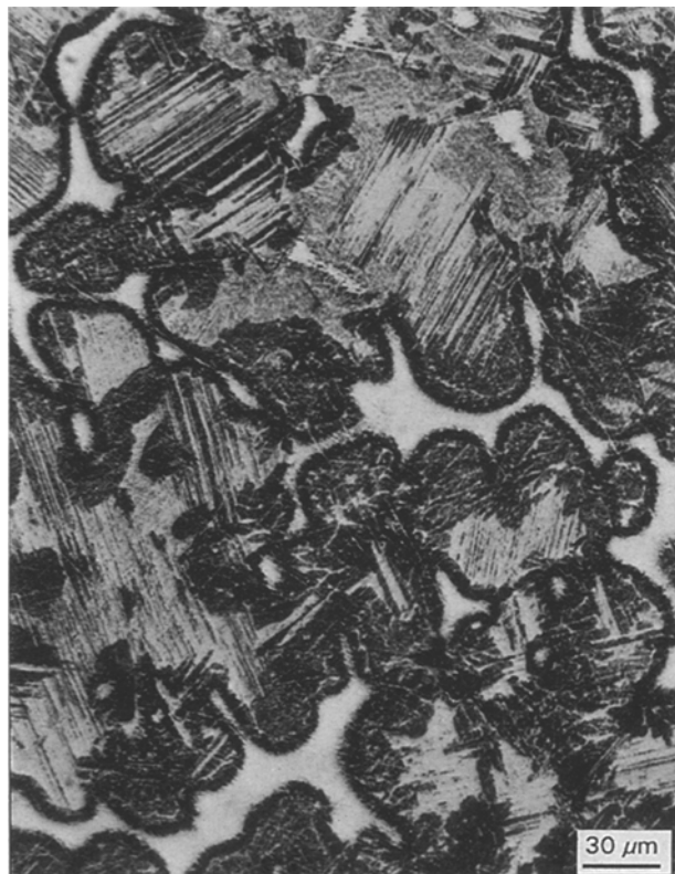
Figure 1 Microstructure of the studied alloy, Ti-50Al (at %)
